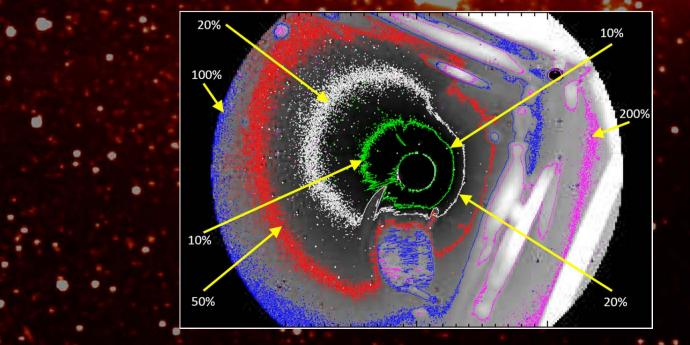
Testing shows SCOPE is performant with stray-light requirement (<20% of F+K-corona) out to ~15Rs in the region away from the spiders (there are clear limitations imposed by the facility).
