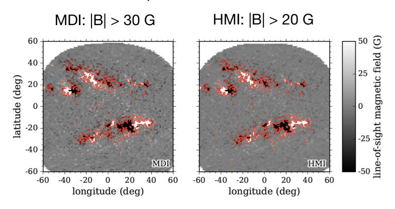
Different thresholds for different instruments (which have different sensitivities to the magnetic field) to make the masked areas the same.
